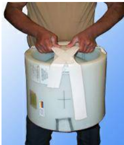
Figure 3-18: Incorrect phantom transportation
