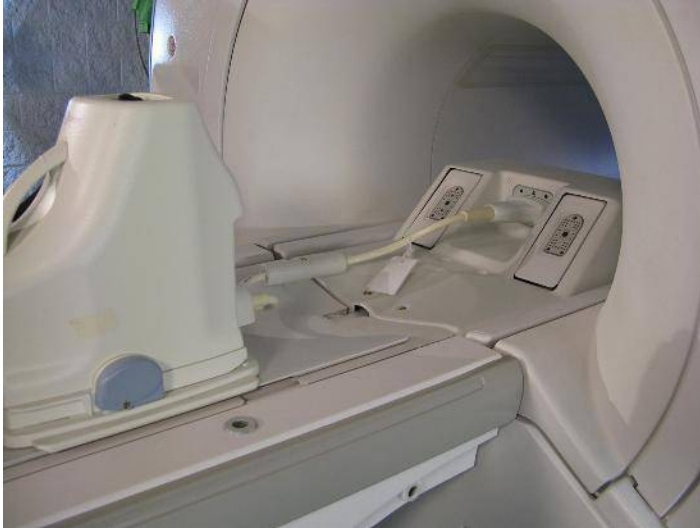
Figure 2-55: Coil cable with no loop
