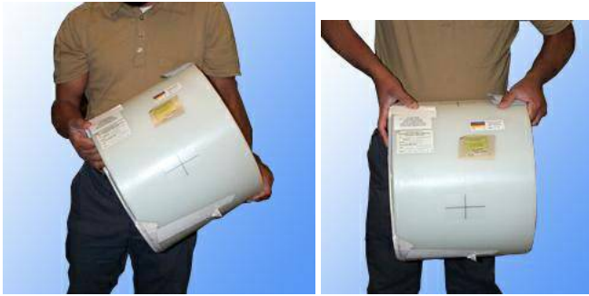
Figure 3-18: Incorrect phantom transportation
