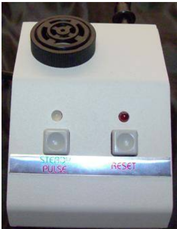
Figure 4-7: Patient Alert control box: Steady/Pulse button on left and Reset button on right
