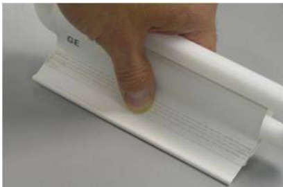
Figure 4-5: Bent strap that more easily slides in the mounting track
